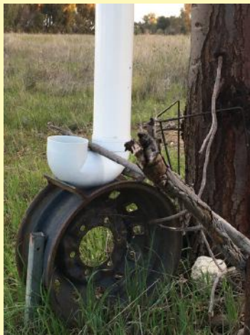
An old car wheel rim provides excellent support, with some bracings welded on
